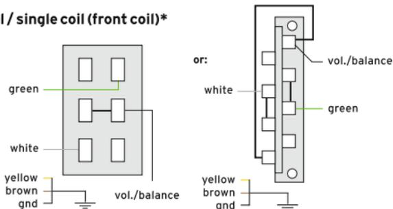
\*) This diagram causes P-bass® type (cross coils in series)/parallel/reversed P-bass® type (cross coils in series) switching with SBC HE/S-4 type pickups.
