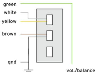
\*) This diagram causes **series/P-bass®** type (cross coils in series) switching with SBC HE/S-4 type pickups.
