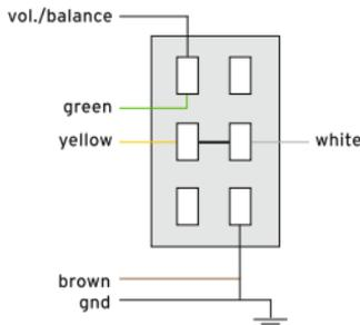
\*) This diagram causes P-bass® type (cross coils in series)/series/reversed P-bass® type (cross coils in series) switching with SBC HE/S-4 type pickups.
