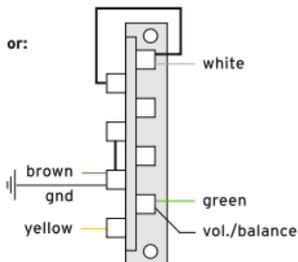
\*) This diagram causes **series/P-bass®** type (cross coils in series)/parallel switching with SBC HE/S-4 type pickups.
